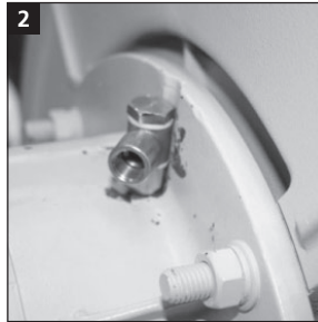
Align the banjo fitting (B) (see picture above) and bolt it with the adapter nipple (A)
