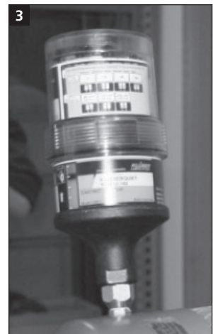
Screw in the pre-assembled cartridge (E, F, H)
